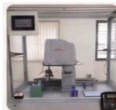
SCARA Robot Cell (High-Speed Assembly Arm 4-Axis)
