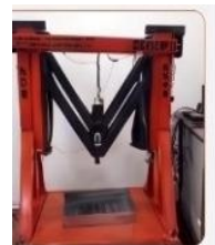
Parallel Kinematic Milling Machine (2-DoF)
