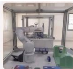
6-Axis Articulated Robot Cell (Flexible Manufacturing)
